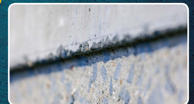
Surface after 10 mm shaving depth
