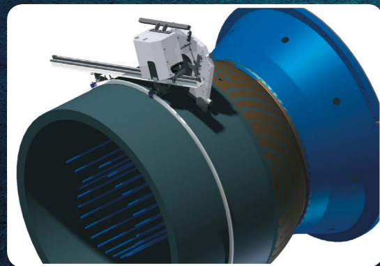
Cutting a pressure raiser
